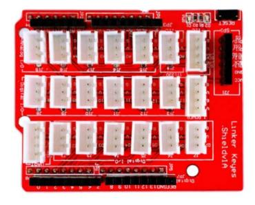
This product also applies for Arduino UNO and its interface definition is exact the same with that of UNO, which helps facilitate connection between Linker Kit series module; This product carries 2.54 interface and supports dupont line.
