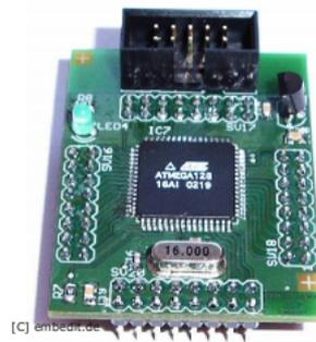
Abbildung 4.5: ATmega128 Platine
