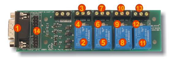
NB. Please ensure the mode selection jumpers are arranged on the board with the metal connection strips positioned horizontally.
