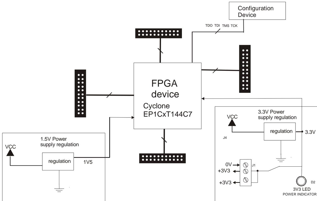
The FPGA Board solution is made up of two parts: The FPGA Board and the CPLD Board. The FPGA together with the CPLD board allow the FPGA to be programmed, and the program to be executed ‘seamlessly’, in the Windows based programming utility Quartus II Web Edition.
